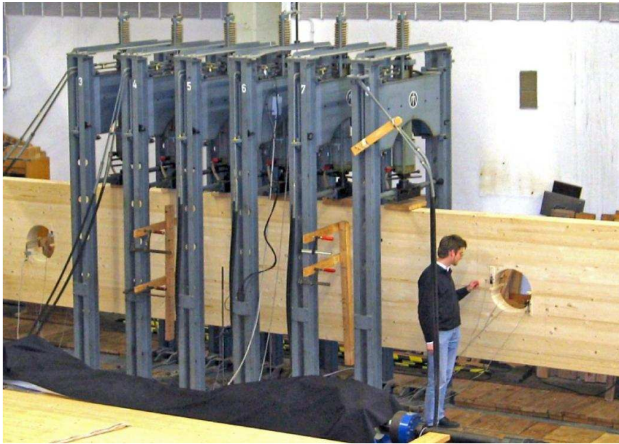
Figure 1.2: Full scale test glulam beam with holes, MPA Stuttgart [32]
