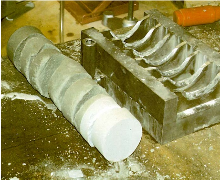
Figure 4.1 Cylindrical specimen of Gotland sandstone after cutting; total length 210 mm, diameter 62 mm. The slices were approximately 30 mm thick.
