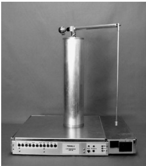
Figure 2.2 The Furuta pendulum
