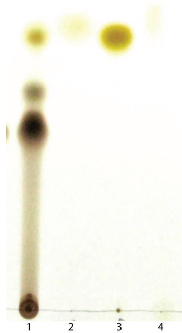
Fig. 1. Thin-layer chromatogram with oxidized p -phenylenediamine (PPD) and reference substances. Solutions were applied on four spots at the bottom line, and eluted with acetone. The four applied solutions are, from the left, oxidized PPD (1), 4-nitroaniline (2), 4,4'-azodianiline (3), and an extract of spot no. 4 from the thin-layer chromatogram (4). Oxidized PPD, solution no. 1, gave four visible spots, of which the second from the bottom may be PPD and polymerized PPD, such as Bandrowski's base.
