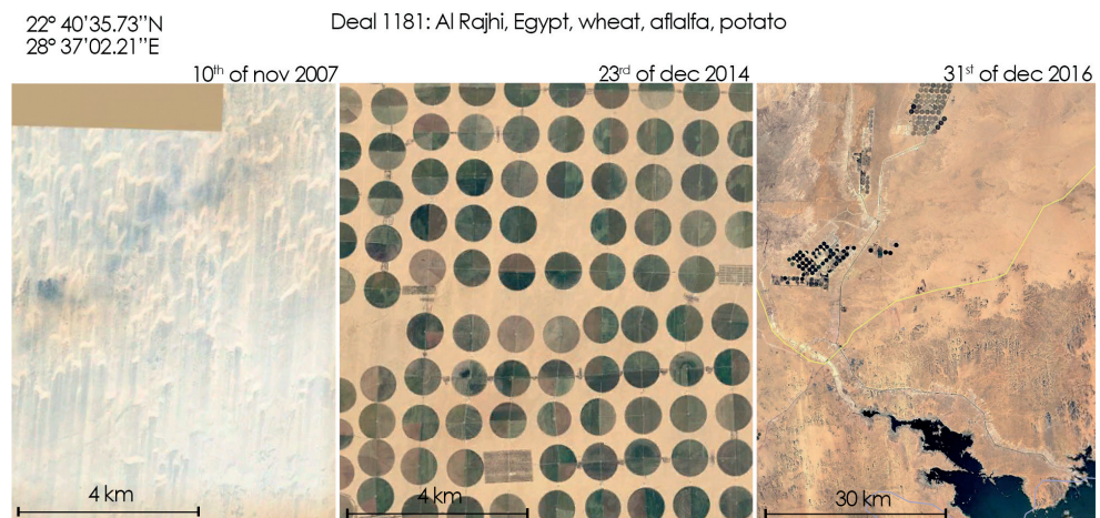
Figure 14. Example of a fully irrigated large-scale land acquisition. Images from Google Earth shows the previous land cover (desert) in 2007 to the left, and the current land use in the middle with wheat, alfalfa, potato irrigated with center pivot systems. Zooming out shows the digging of canals for irrigation purposes in the image to the right.
