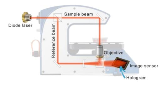
Figure 2. The optical set-up of the HoloMonitor M4.
