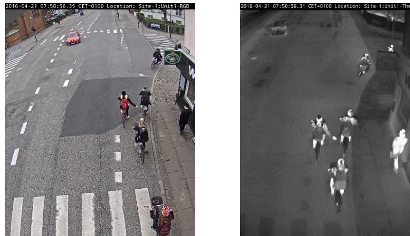
Figure 3. Views of the same traffic scene taken simultaneously with an RGB and thermal camera.
