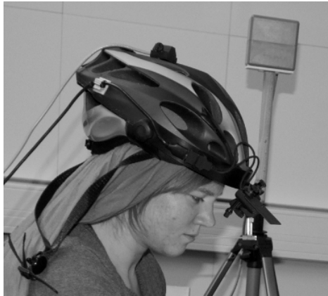
Figure 7: Example of the head-mounted eye-tracker used in Paper I. The device generating the magnetic field is located in the upper part of the figure.
