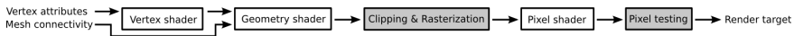
Figure 1: An overview of the pipeline of a modern GPU. White boxes represent the user-programmable stages and grey boxes represent fixed functionality.
