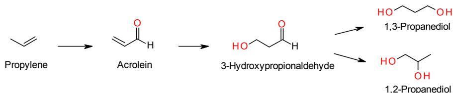
**Figure. 4.2. Degussa process for production of 1,3-propanediol from propylene via 3-hydroxypropionaldehyde**
