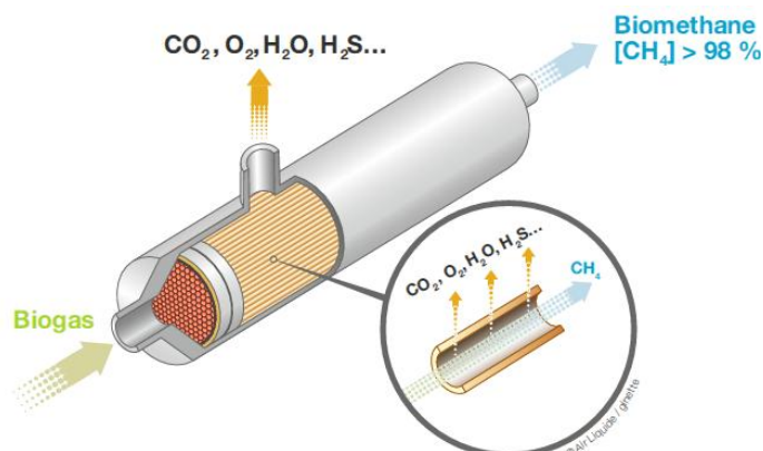
Figure 11 Illustration showing the separation involved during upgrading of biogas with membranes. Image from Air Liquide.
