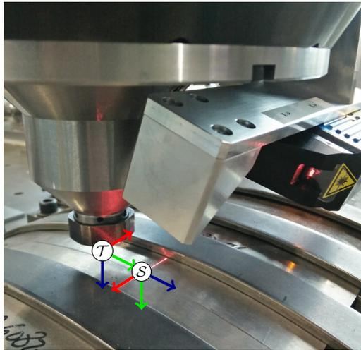
**Figure 14.1** Coordinate frames  $(x, y, z) = (\text{red}, \text{green}, \text{blue})$ . The origin of the sensor frame  $S$  is located in the laser plane at the desired seam intersection point. The tool frame is denoted by  $\mathcal{T}$ .
