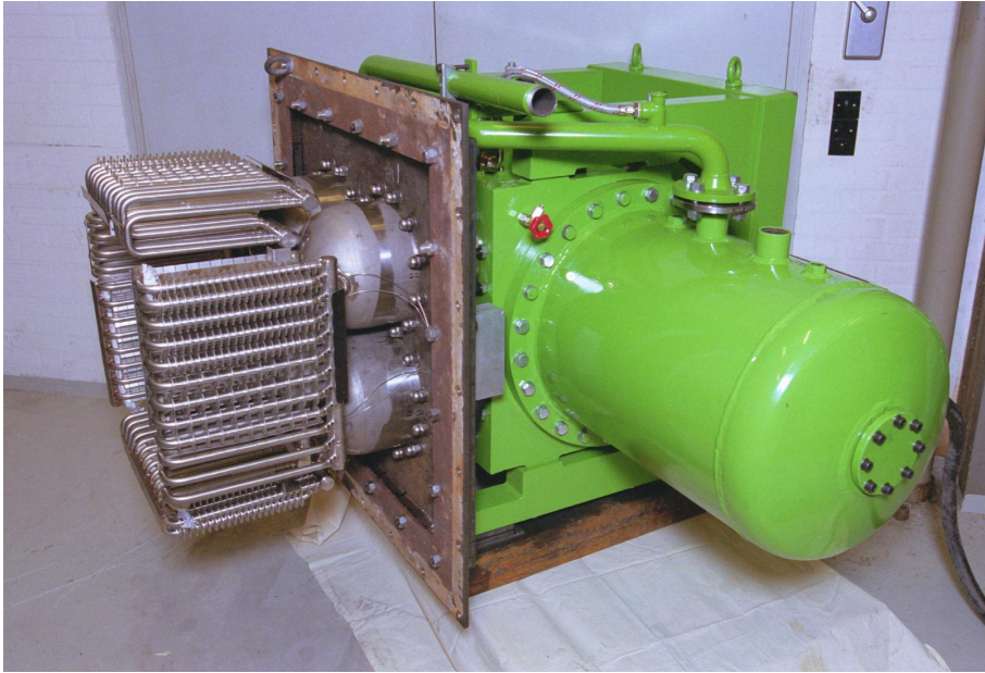
Figure 1 Photo of the SM3D Stirling engine that will be used in the project
