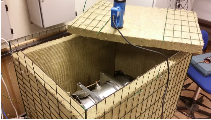
Figure 3.12: Machine mounted inside the heat box for the dynamic on-load tests
