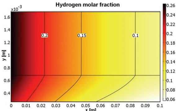
Figure 9: Molar fraction of hydrogen within the fuel channel (top) and anode (bottom).
