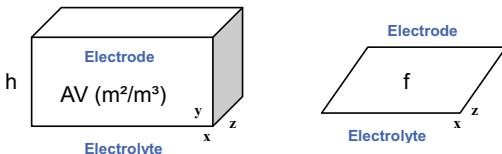
Figure 3: Sketch over the concepts (source term, to the left, and interface condition, to the right) to define active area for the electrochemical reactions
