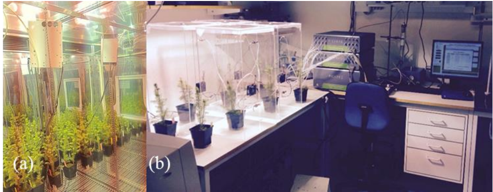
Figure 4. a) Seedlings were kept under controlled moisture, CO 2 concentration, and light intensity. b) 13 C pulse-labelling using plexiglass boxes connected to Picarro analyzer (Paper V).
