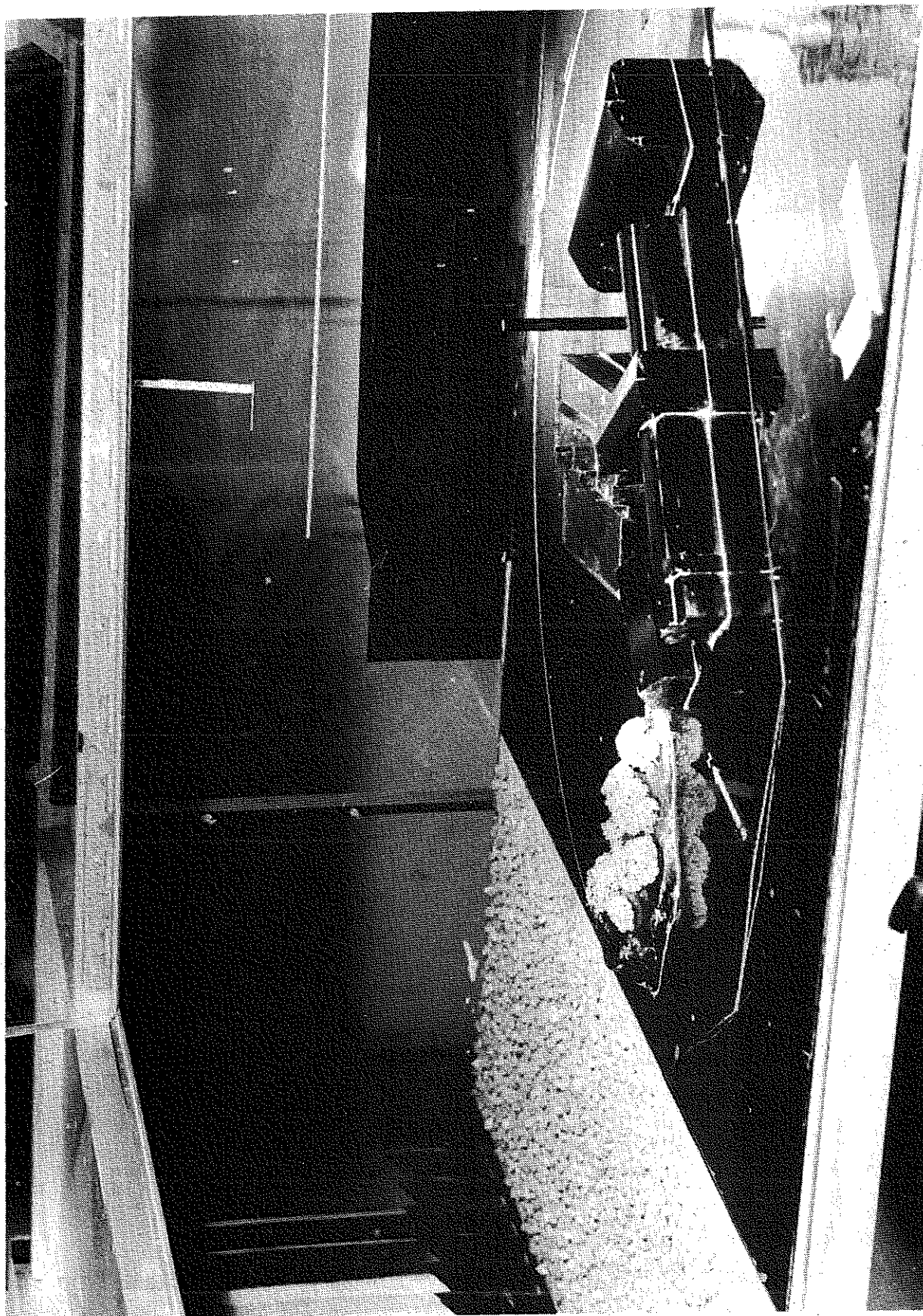
Figure A3c. The model in the test section of the FFA building aerodynamics-tunnel
