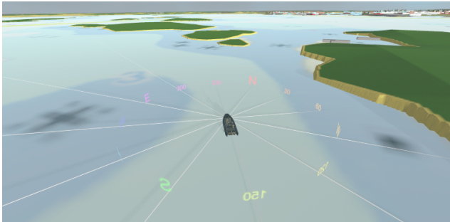
Figure 53: TeV : The own ASV is situated in front of the virtual user, as the user was paragliding after the boat. The dark blue in the sea chart indicates a dangerous area with a bottom depth less than 3m. In TeV, the user can easily get a feel for the own ASV's size compared to the passage between the shallow areas.
