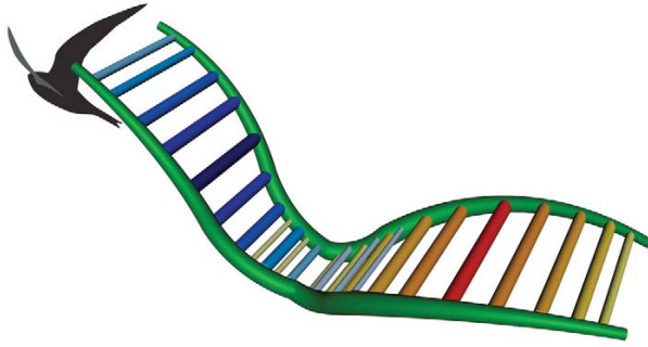
Fig. 10. Three-dimensional wake structure of the swift in cruising flight. The image frame is as if the bird flew obliquely from right to left and slightly into the paper, leaving the trace of one wingbeat in still air, starting at the upper turning point. Green tubes show the wingtip vortices, cylinders in shades of red are spanwise vortices with positive circulation and cylinders in shades of blue have negative circulation. The colour intensities and tube diameters are proportional to the strengths of each component. The geometry is deduced from a combination of wingbeat kinematics and streamwise plane section data.
