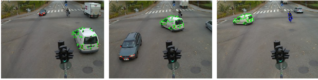
Figure 5. Three frames from the video. The pose for the three vehicles has been calculated for the frames where the vehicles are visible.
