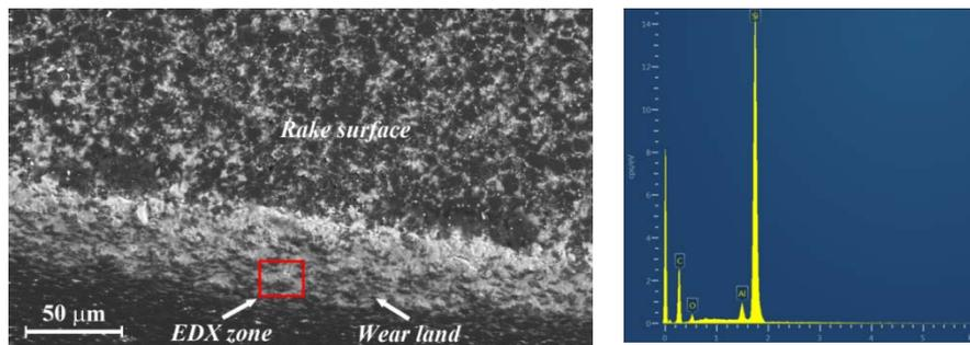
Fig. 18. (a) SEM close-up view of worn D-Co insert ( $v_c = 400$  m/min) after etching, (b) EDX spectrum for layer adhered to the wear land.
