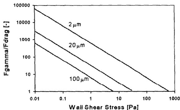
Fig. 3. Force ratio diagram. By moving horizontally in this plot the scale can be increased in both size ( $D_p$ ) and time (reducing the continuous phase flow velocity generating the wall shear stress) while maintaining an equivalent force ratio on each scale.
