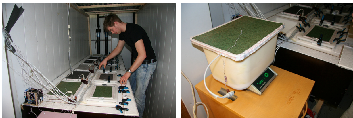
FIG 3. Picture of the test rig in the cold room, left. The boxes stood on a plate that was heated to normal indoor temperature of 20 °C. The boxes closest to the wall were used to measure water vapour permeance/resistance. On the other boxes, the row to the right, the underlay samples were attached to removable plastic lids for measuring moisture uptake. The weight changes of the boxes during the test period were measured by use of a balance as shown on the picture to the right.
