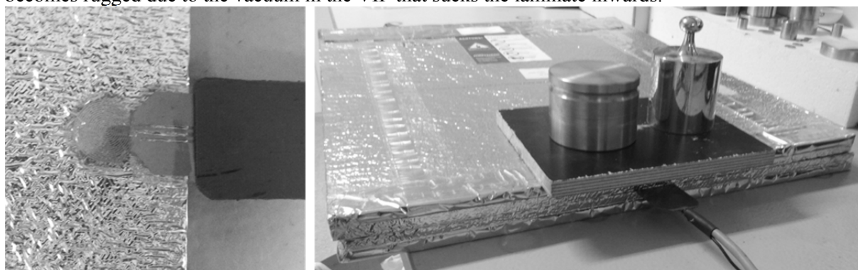
FIG 1. TPS sensor on a functioning VIP (left) and measurement setup with the sensor clamped between two VIPs (right). There is a pressure of 4.7 kPa applied on the upper sample to increase the contact with the sensor.
