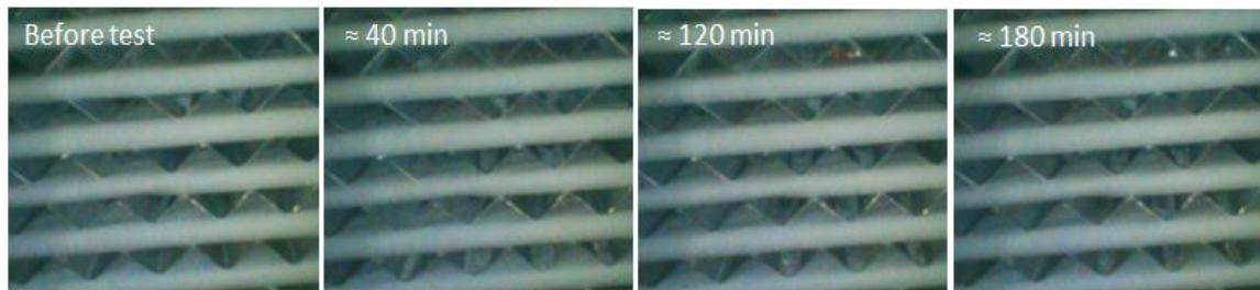
FIG 7. Photographs of frost formation in the hydrophobic ERV.
