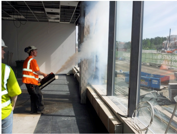
FIG 4. Air leakage testing of window details with smoke.
