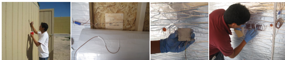
Figure 3: Installing temperature and heat flux sensors. Left to right: temperature sensor on exterior wall, heat flux sensor on interior side of OSB and thermocouple array through assembly, and installing heat flux sensor on reflective insulation with reflective tape.
