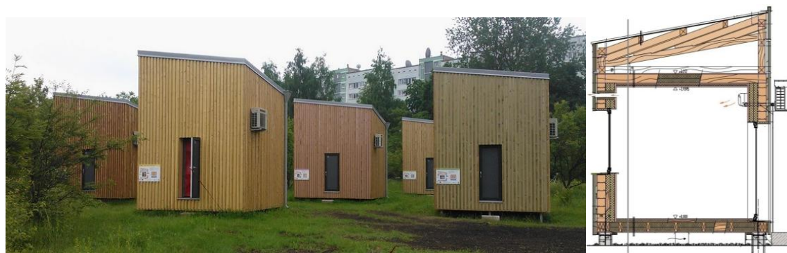
FIG 1. On the left: The test stands of houses. On the right: A cross-section of one test stand
