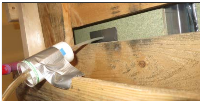
FIG 3. Sampling of air from inside a CLT element, via a hole drilled in the particleboard on the edge surface of the element.
