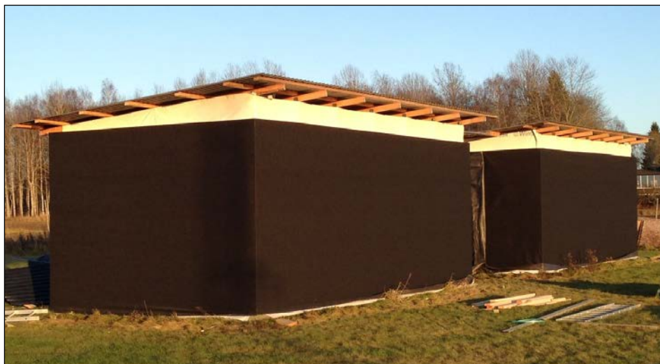
FIG 3. Field test at Ås. Two identical test-houses (7.0 m x 3.6 m x 2.2 m internal measurements).
