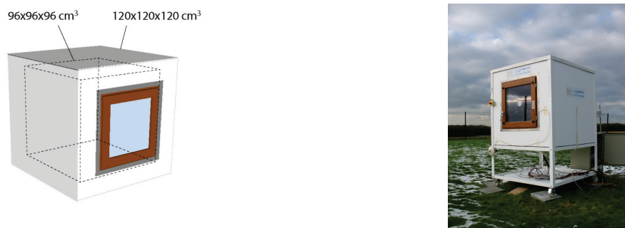
Figure 4. The test box from the IEA Annex 58 (2013), Left: design, Right: as built
