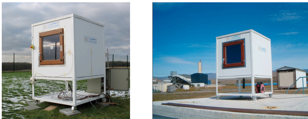
FIG 4. Test box during winter at the measuring site at BBRI, Belgium (left) and during summer at the Plataforma Solar de Almeria, Spain (right).
