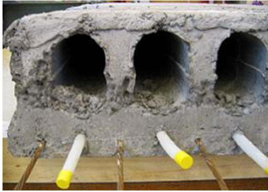
FIG 2. Concrete hollow deck with integrated PEX pipes
