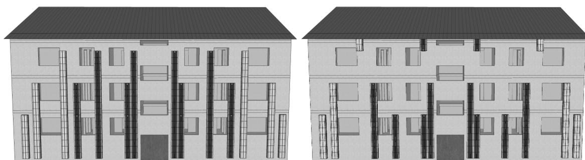
FIG 7: Solution for the air ducting on the façade with limited space between the windows: connection of two rooms with one duct (left) and with air ducting through the attic and the basement (right)
