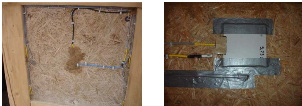
Fig. 4. Outer sensors at layer 1 beneath the outside rendering (left) as well as Temperature sensor, heat flow wafer and humidity sensor on barrier layer 3, beneath internal insulation on the second insulation board layer (right).
