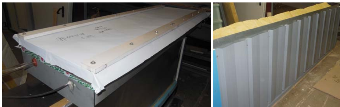
FIG 1. Measurement of the joint between two vapour barriers (left) and between slab and wall (right)
