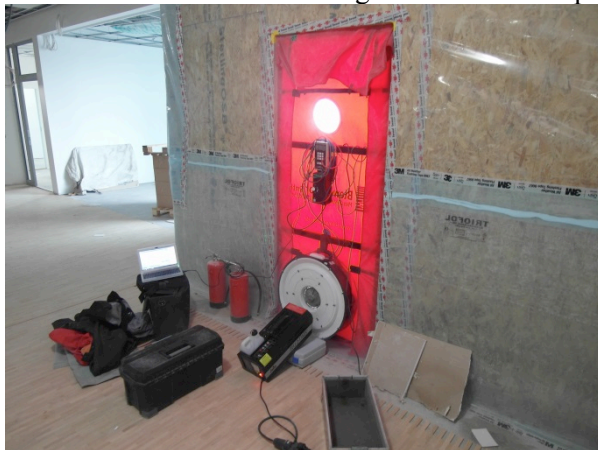
FIG 3. Blower-door equipment attached to a provisional wall with a smoke machine placed at the fan inlet.
