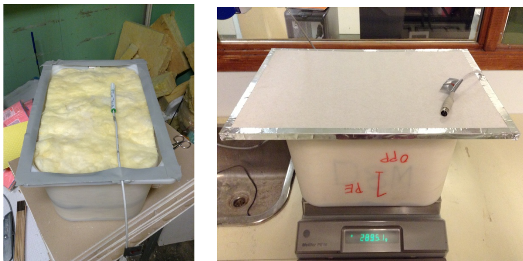
FIG 1. Test box with RH/T-sensor before mounting of SVB (left) and after mounting of SVB and gypsum board.
