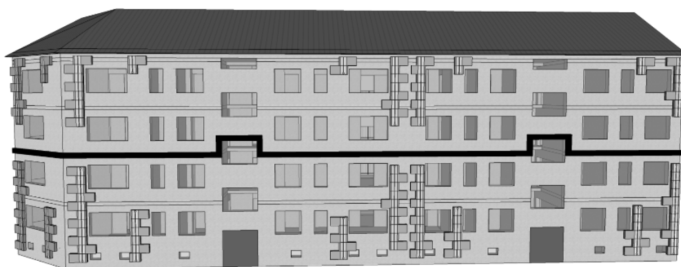
FIG 8: Fire barrier and separated supply air ducting through the attic and the basement, exhaust air ducts installed subsequently in existing chimneys
