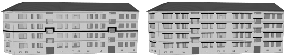
FIG 3: Additional fire protection for class 4 buildings with fire barrier above every second floor (left) and with window lintel protection (right)
