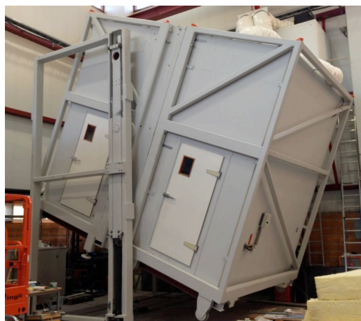
Figure 2. The guarded hot box test facility used for the measurements
