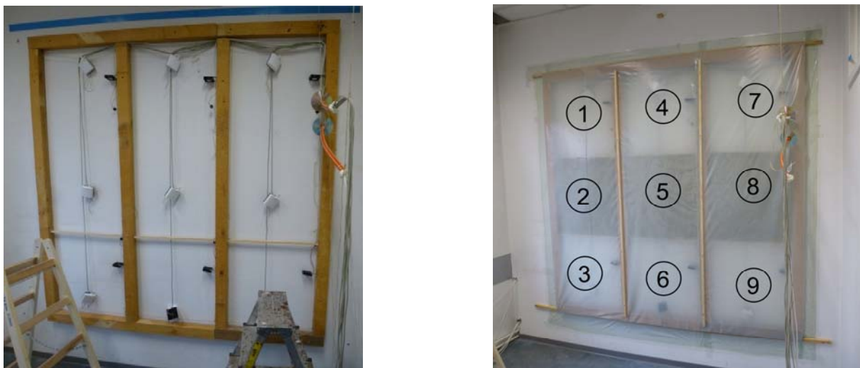
FIG. 2 facing formwork in laboratory test rig; left without foil, right with foil and indication of fields
