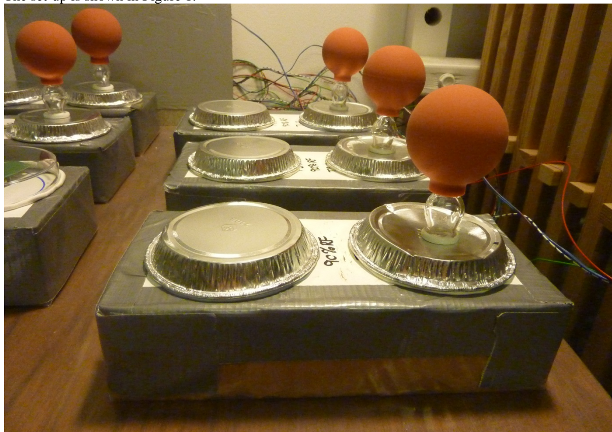
Figure 1. Experimental set-up showing moisture hoods sealed at the edge to the surface of bricks wrapped in PE-foil. Two experiments are conducted at the same time; one with under pressure (with suction device) and one without pressure difference.
