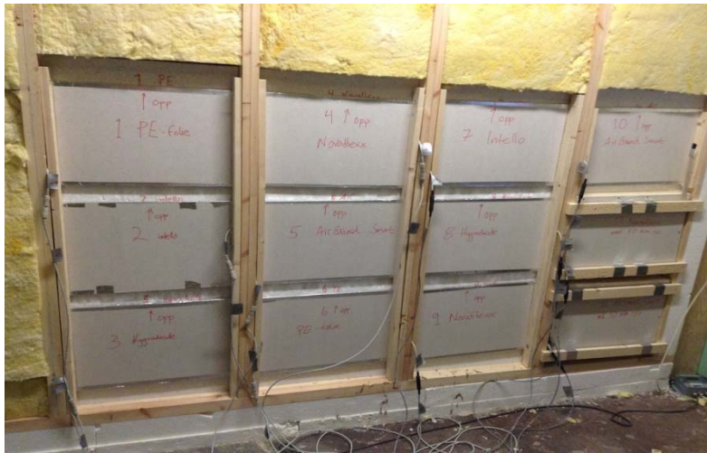
FIG 2. The experimental set-up showing the 10 test boxes installed in the wall, seen from the warm side.
