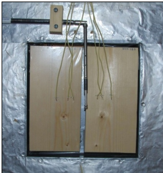
FIG 1. Samples mounted in housing. View Samples (covered left, uncovered right) and thermocouples mounted in the ceiling of a well controlled climate chamber. In center the air speed meter is placed.
