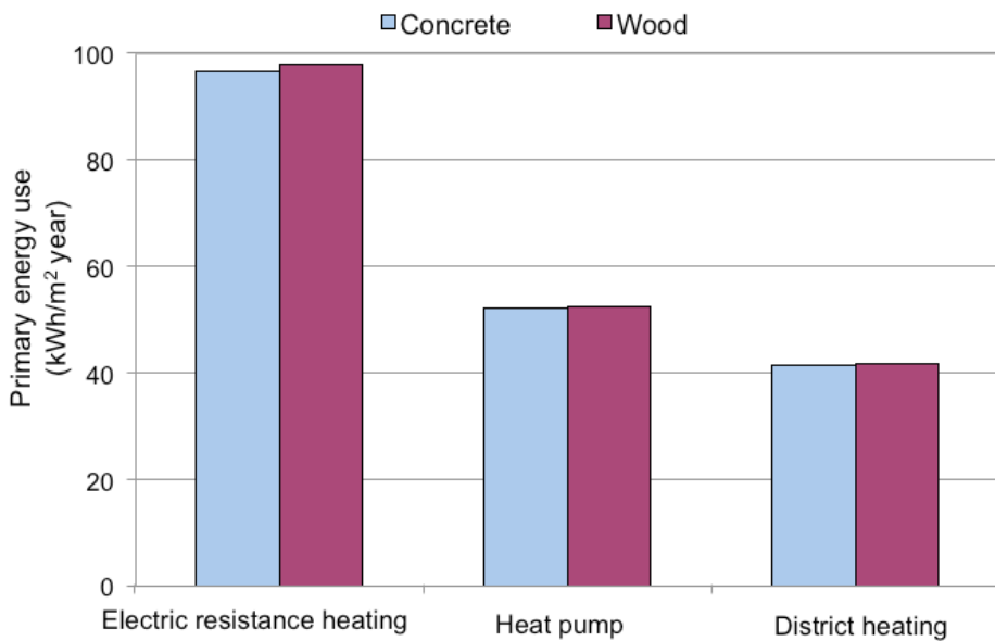
Fig. 3. Annual primary energy use for bio-based heating and ventilation of a conventional house with electrical heating, a bedrock heat pump or district heating using combined heat and power production, in units of kWh per square meter heated building area. The house is assumed to be built in Växjö with a concrete or wood frame. (Adapted from: Dadoo, A., Gustavsson, L., & Sathre, R., 2012)
