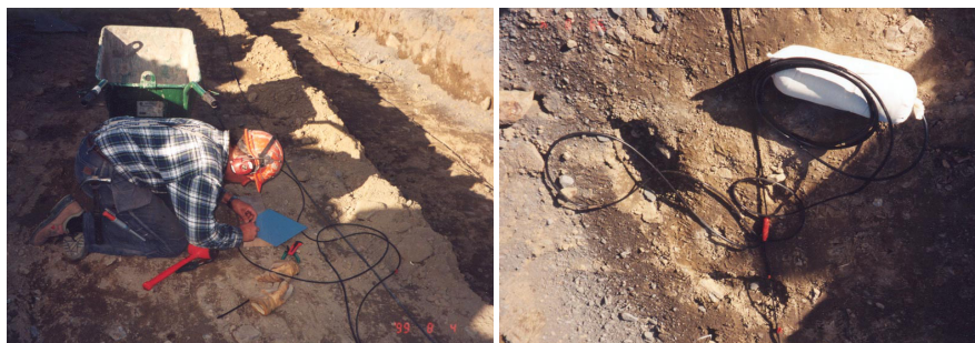
Figure 16. Installation of electrodes at Sädva. Both steel plate electrodes (left) and non-polarisable copper-copper sulphate electrodes pre-packaged in cloth bags with bentonite (right) have been installed.
