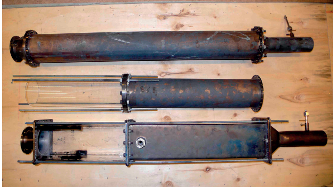
Figure 5.3: Three burner confinements used in atmospheric testing. Burner attaches from the left with quarl, which interfaces to the combustion liner. Liners terminate at right with a contraction and exhaust tube where the emission sampling port is located.
