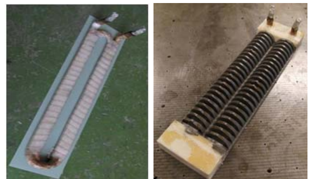
Figure 5. Left: Coil design, right: finished inductor, moulded in SM 2 C
