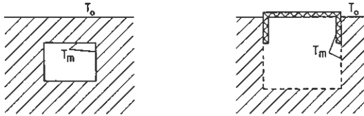
Figure 12.1. Steady-state thermal process around a ground heat store with constant temperature T_m at the storage boundary. The temperature at the ground surface is T_0 .
