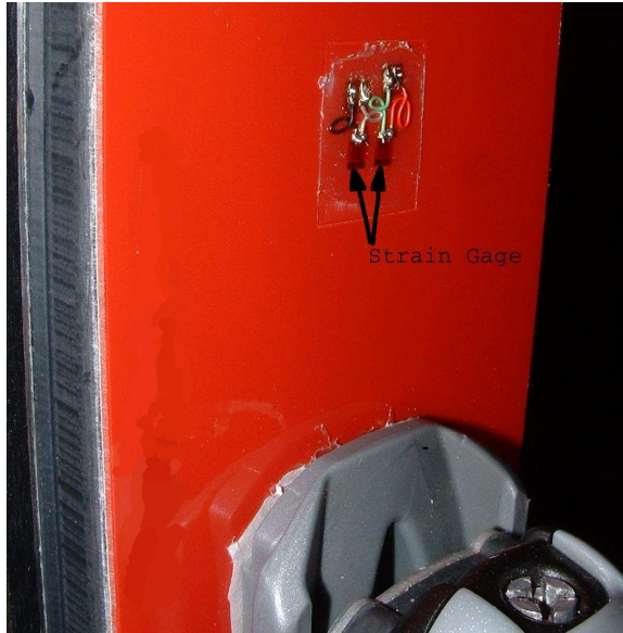
Fig. 2. The strain gages mounted on the ski.
