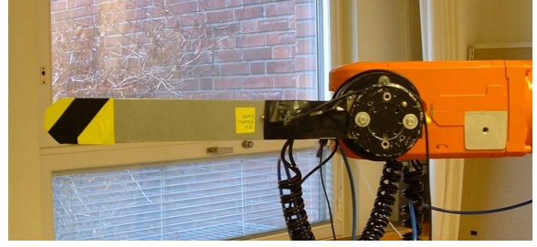
Fig. 3. The beam connected to the end-effector of the robot manipulator.
