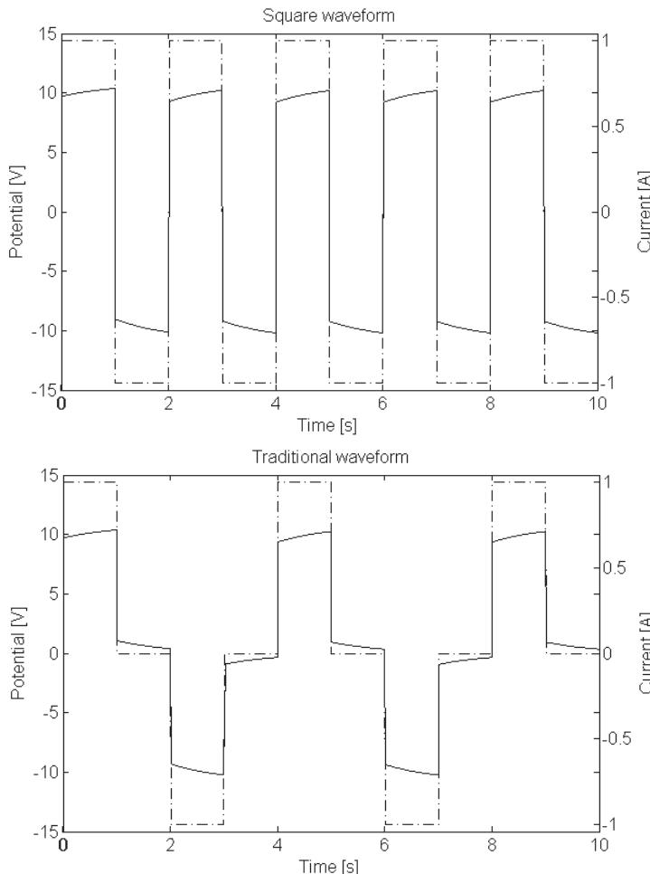
*Fig. 1: Modelled waveforms using superposition of step response. The step response is calculated for a homogeneous half space ( $\rho = 50 \Omega m$ ,  $m_0 = 100 mV V^{-1}$ ,  $\tau = 1.0 s$  and  $C = 1.0$ ). The upper diagram shows the square waveform without off-time and the lower diagram shows the traditional waveform. Potential is drawn as solid and current as dash-dotted line.*
