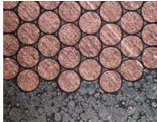
Figure 2: Microscopic picture of the winding and the core material. The wire is 0,7 mm in diameter.
