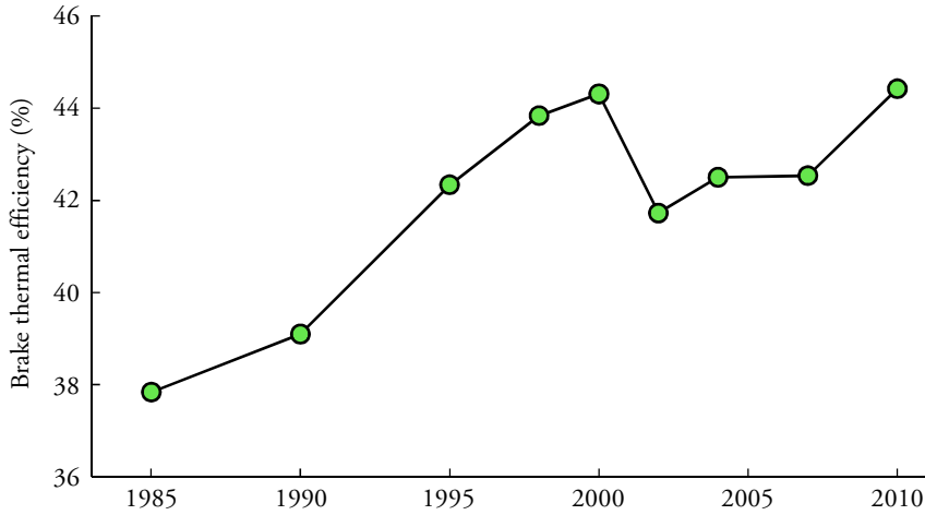
Figure 1.1: Engine brake thermal efficiency over the years at cruise load conditions, adapted from data in [3].
