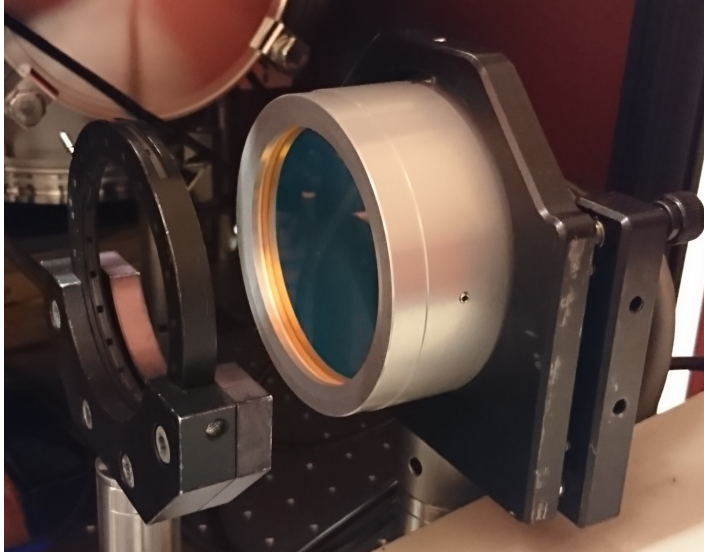
Figure 3.3: A photo of one of the DMs installed at the high-intensity XUV beamline.
