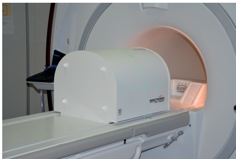
Figure 1. The commercially available phantom from Spectronic Medical AB is designed to assess geometric accuracy. It was placed on the MRI table without table top. Lines on the phantom surface were used to align the phantom using the built in laser positioning system on the MRI.
