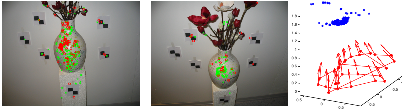
Figure 5.4: The triangulation problem. Two images with points used for calculating the reconstruction to the right. Green points (inliers) are used for the triangulation while red points are detected as outliers.
