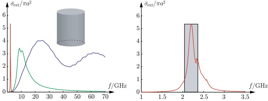
Figure 1: The averaged extinction cross section  $\bar{\sigma}_{\text{ext}}$  in units of  $\pi a^2$  as function of the frequency for a Lorentz dispersive cylinder with volume-equivalent sphere of radius  $a = 1$  cm. The right figure is a close-up of the 2 GHz peak and illustrates the physical limitations presented in Sohl et al.[2].
