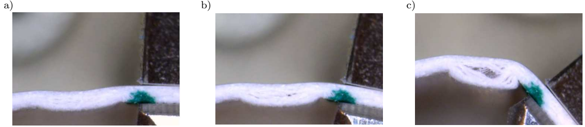
Figure 6: Folding of creased paperboard. The bending angles are approximately (from left to right) 10, 20 and 60 degrees.
