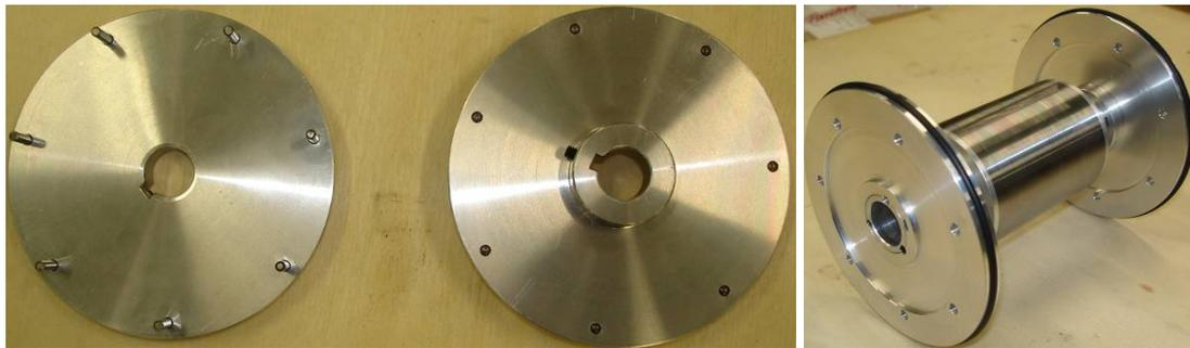
Figure 4.23 Prototyped parts: transmission disks (left) and rotor attached to the inner transmission rings with o-ring.
