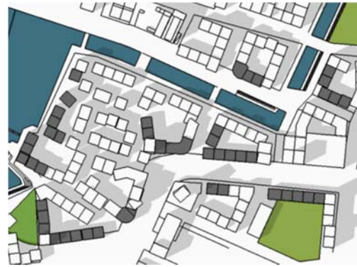
Fig. 13. Shade patterns in central Nyhamnen on 21 st March/September at 9 a.m. and on 21 June at 3 p.m. The dark buildings have been lowered to 5 storeys to allow for more solar access in the courtyards and in the street.
