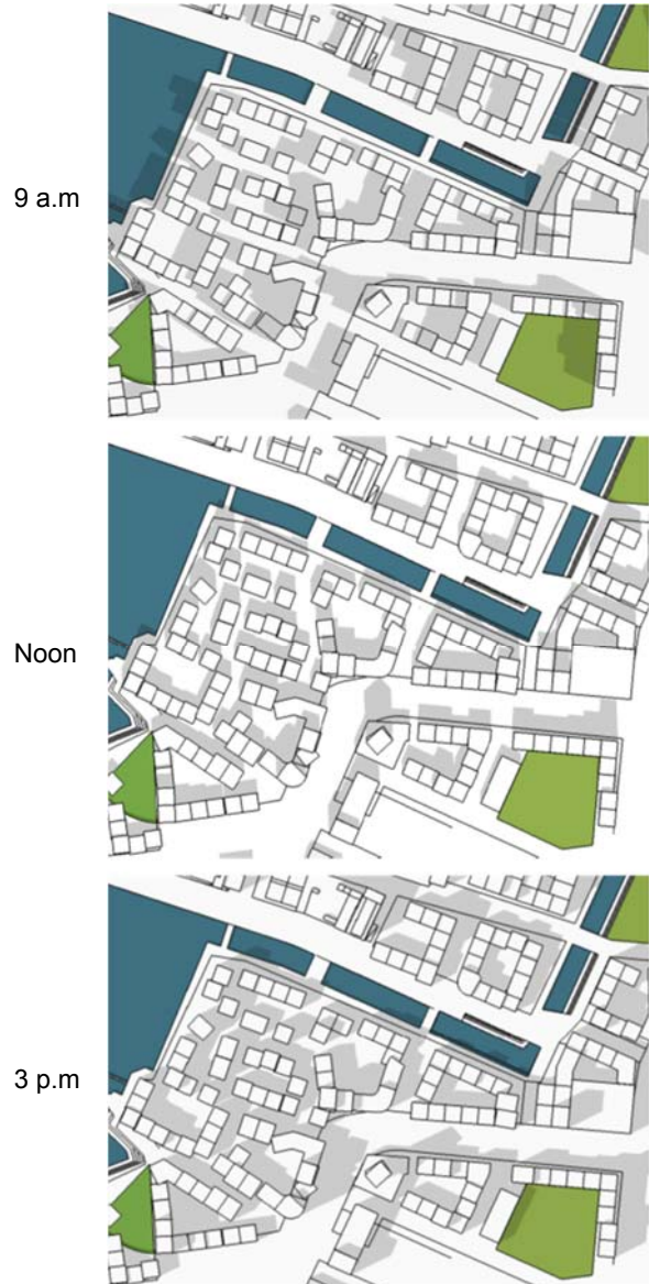
Fig. 10. Shade patterns in central Nyhamnen on 21 st June at 9 a.m., noon and 3 p.m.
