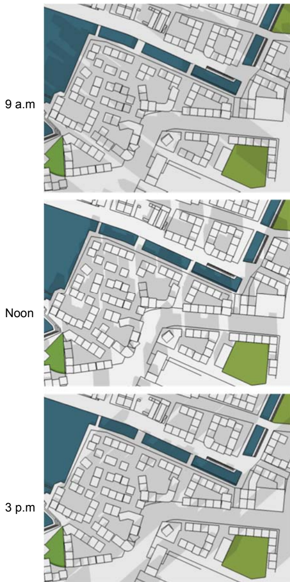
Fig. 9. Shade patterns in central Nyhamnen on 21 st March/September at 9 a.m., noon and 3 p.m.
