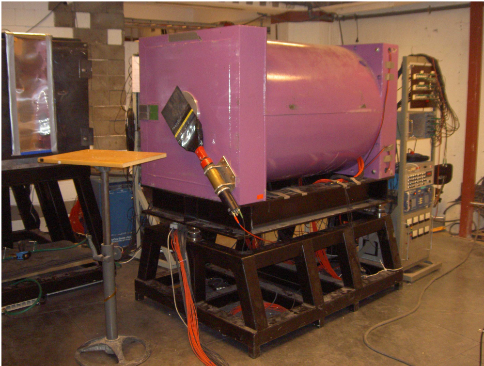
Fig. 6. The CATS detector (on loan from the University of Mainz, Germany) shown in situ at MAX-lab. The detector itself is encased in lead shielding, and the resulting canister is mounted on a heavy steel frame. The steel frame sits on airpads which allows for the entire apparatus to be positioned with relative ease. The other two detectors are very similar.
