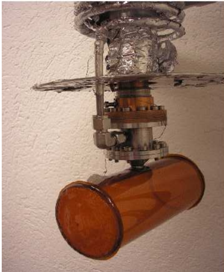
Fig. 5. The liquid deuterium target cell. The cell is 68 mm in diameter by 150 mm in length. The symmetry axis of the cell lies along the photon-beam axis.
