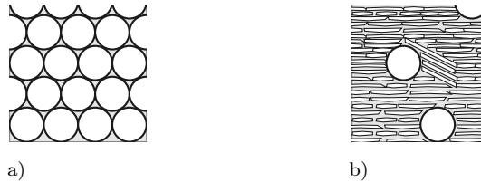
Figure 4.1: Idealisation of a granular and clayey soil where white represent solid particles and grey fluids. a) granular soil. b) clayey soil.
