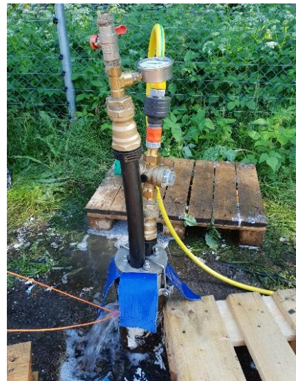
Figure 6 – Installation of the coaxial collector with a flexible outer pipe in the 200-m deep borehole for in-situ tests.
