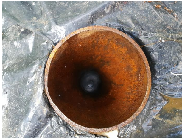
Figure 4 – Photograph of the 200-m deep groundwater-filled borehole used for comparative testing of the ground collectors.
