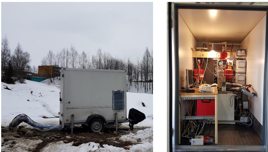
Figure 3 – Photographs of the thermal response test rig.
