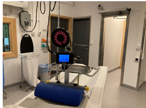
Figure 6 Infrared camera mounted on the PET/CT table and an infrared reflective marker block that is fixed to the patient chest.
