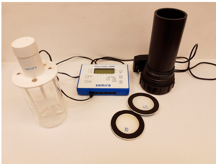
Figure 6 Photo of the Kemira Flocculator 2000 (Helsingborg, Sweden) and disc filters used during this study ( Paper I ).
