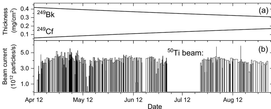
FIG. 1. (a) Chronological evolutions of isotopic thicknesses of  $^{249}\text{Bk}$  and  $^{249}\text{Cf}$  with an average total thickness of  $0.48(5) \text{ mg/cm}^2$  during the irradiations with the  $^{50}\text{Ti}$  beam with an energy of  $E_{\text{lab}} = 281.5 \text{ MeV}$  in the middle of the target. (b)  $^{50}\text{Ti}$  beam current on the target averaged over time of each set of the irradiation.
