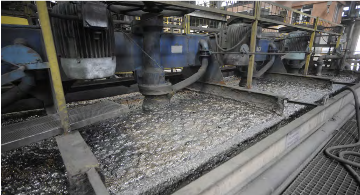
Figure 1.3 Flotation process to obtain metal concentrate.
