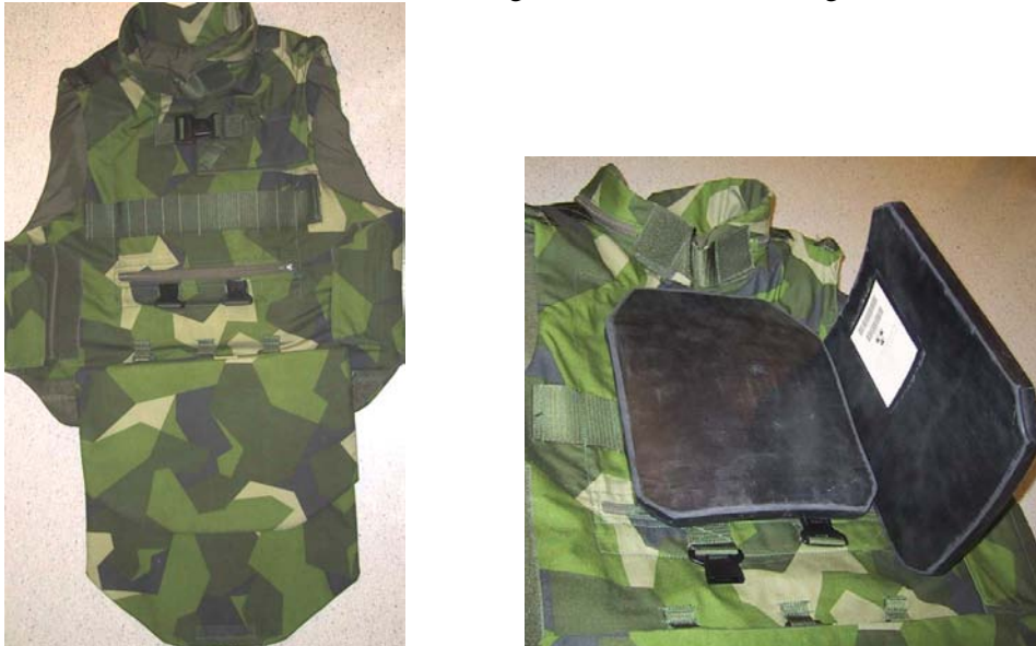
Figure 1. Body armour used (left). Hard back and front plates when not inserted (right).
