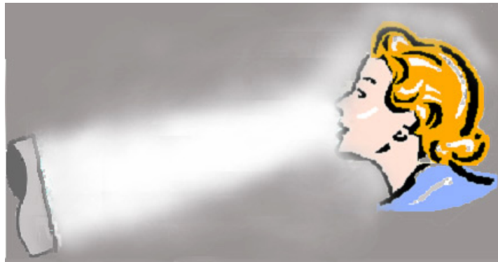
Figure 1. The principle of personalized ventilation: small amounts of cool, dry, and clean air should be supplied directly and gently to a person's breathing zone and be easily controllable by the individual.
