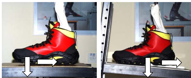
Figure 4: Test of slip resistance of a hiking boot during backward movement, at surface angles of 0^\circ and 5^\circ .
