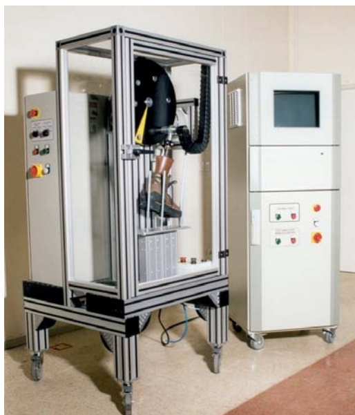
Figure 1: The thermal foot manikin system comprises three components: the Gait Simulator (left), the Sweating Thermal Foot Manikin (attached to the flywheel of the gait simulator), and the Control Unit (right).
