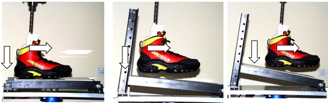
Figure 3: Test of slip resistance of a hiking boot during forward movement, at different surface angles ( 0^\circ , 5^\circ and 10^\circ ).
