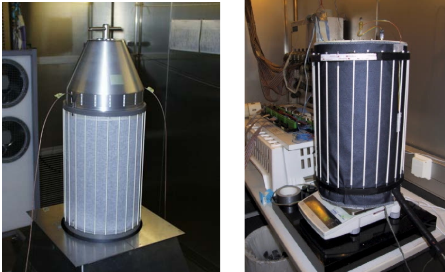
Figure 1. The sweating cylinders of EMPA (left) and SWL (right) with spacer rings.
