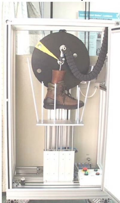
Figure 3: Simulation of gait is achieved by the combined action of the flywheel and pneumatically driven platform (see text for details).
