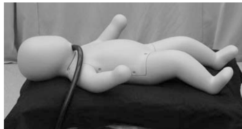
Fig. 1. Picture of the newly developed infant thermal manikin. Whole body of the manikin can be controlled at the same time and each part can be also regulated separately at the desired level through two modes.
