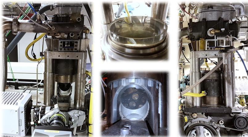
**Figure 3.3.** Images from an optical engine converted according to the Bowditch design. In this case, drop-down liner is used, a flat-top piston and three liner windows are used to obtain lateral access inside the combustion chamber
