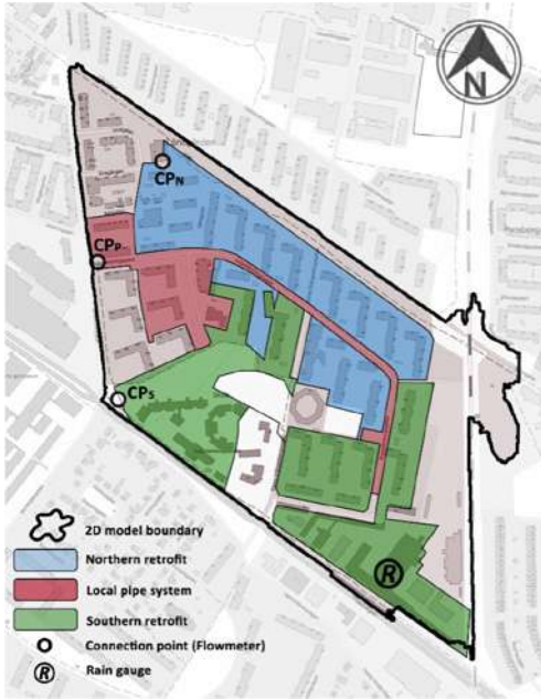
Figure 2. Catchments in Augustenborg and their drainage systems; adopted from Haghighatafshar (2019).
