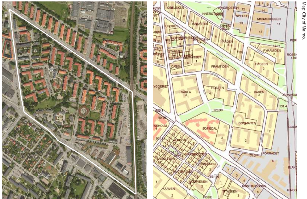
Figure 1. Augustenborg is built as a neighbourhood unit which follows the “houses in the park” urban development tradition which dispenses with visible borders as far as possible between the land linked to apartment buildings and their surrounding parkland, streets and public land for school, etc. But plot boundaries, as shown in the map to the right, add a complexity that any stormwater system needs to tackle, as water does not respect property boundaries but moves according to the topography from higher to lower lying points. The stormwater system is connected to the public drain network in the west, marked with a blue dashed line. All excess stormwater will be led here.
