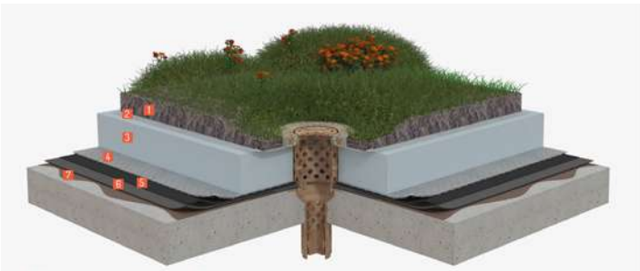
The Green Roof Handbook provides good detail on how to construct difficult parts of green roofs. This shows a safe and waterproof drain installation. Drains are always needed on roofs to remove excess water so that it does not leak down into the building below.
