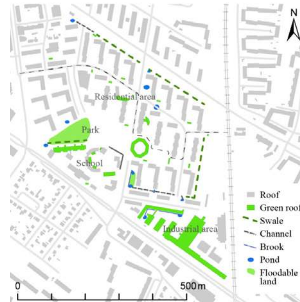
Figure 1. Situation plan of Augustenborg stormwater system, including green roofs, swales, channels, brooks, ponds and floodable land. Illustration by Johanna Sörensen
